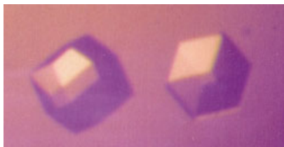
FIGURE 4 The 2.1 Å diffracting crystals of ramoplanin A2.
