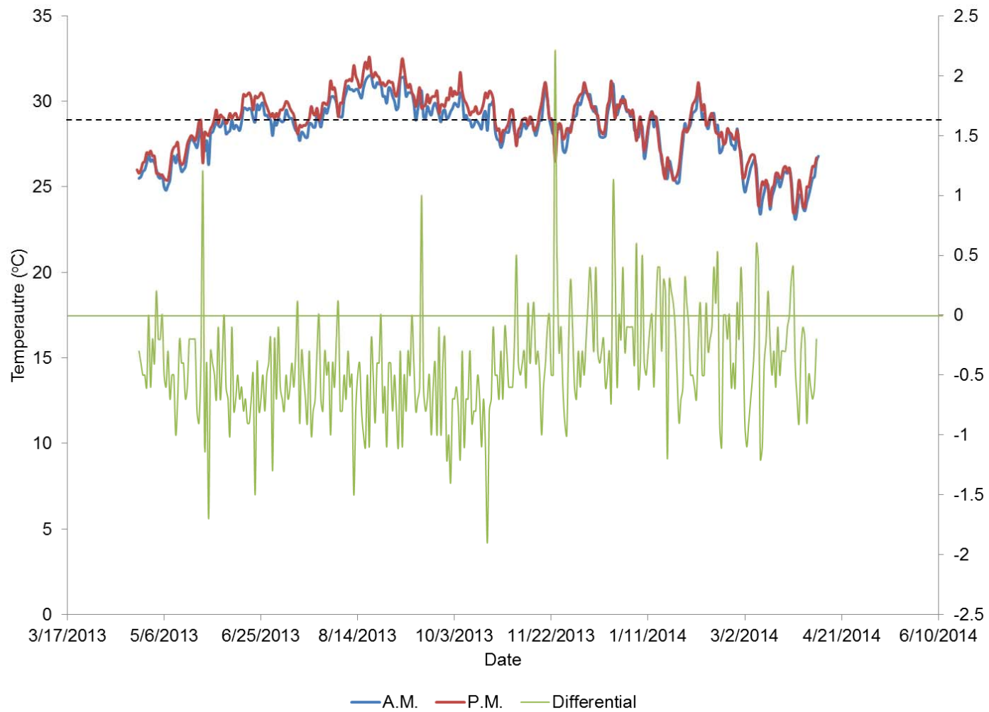
Figure 2. Temperature in the commercial demonstration system throughout the grow-out period. Black horizontal line denotes the set point for the solar panel for either radiant cooling or solar heating. Green horizontal line denotes the zero differential between morning (9 a.m.) and afternoon (4 p.m.) temperature in the system.
