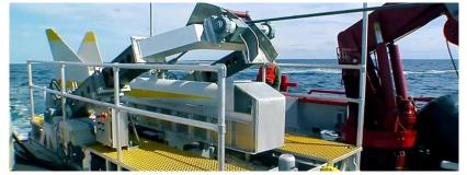
Raytheon photo - Raytheon and FAU Harbor Branch perform developmental testing. The Littoral Combat Ship Variable Depth Sonar deployed and recovered at sea.
