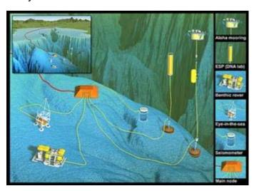
The Monterey Accelerated Research System (MARS), is a cabled seafloor network which will allow instruments, such as MEITS to be connected continuously to shore from 3000ft. deep in the Monterey Canyon.
