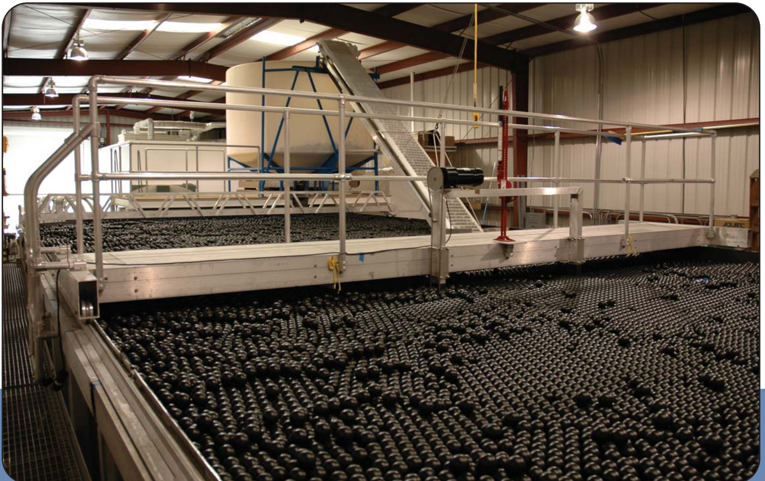
This view of the surface of the test facility tank shows plastic balls deployed from a main hopper above the tank to control the amount of ambient light that penetrates into the water below.
