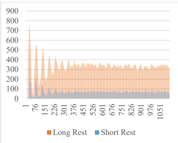
Figure 31: Number of trucks in rest at Rest Area 19 with 55 mph cruise speed result
