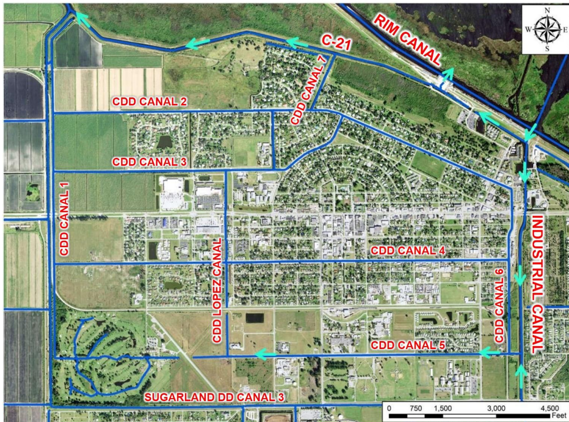
Figure 48. Local drainage canal system in the City of Clewiston (CCD=Clewiston Drainage District).
