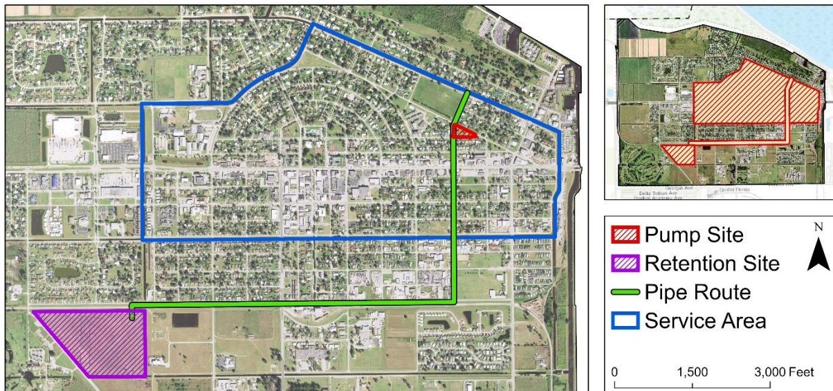
Figure 71. Proposed site layout of flood control pump station for eastern Clewiston, FL
