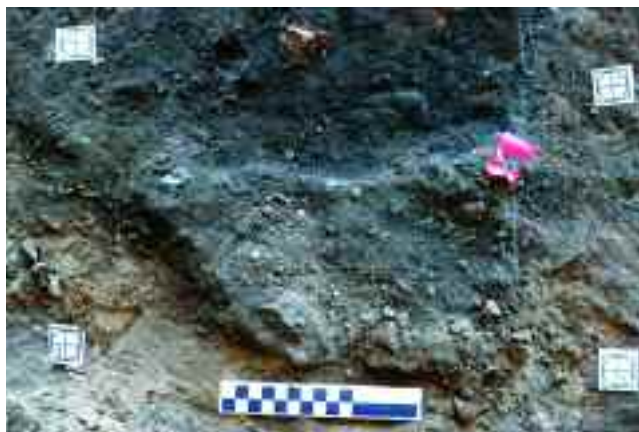
Figure 4: A plan photograph of a feature (a burned area) showing targeting chits that will be shot by the total station. This particular set-up is for a photograph that will then be rectified and built into our GIS.
